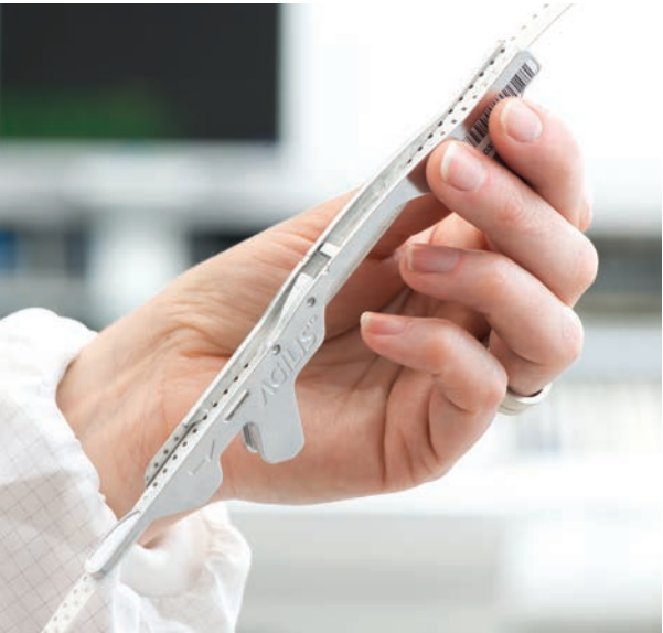
The compact Agilis tape feeder is extremely fast to load.
