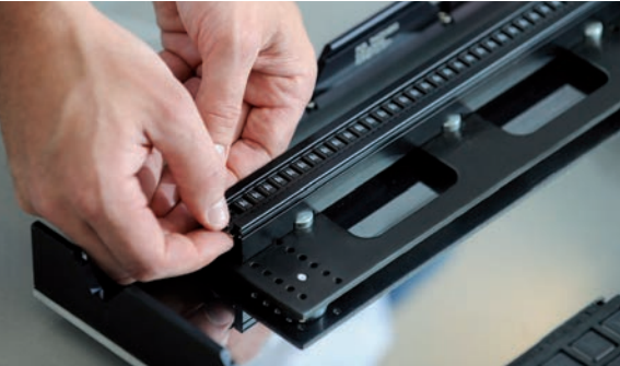
Handle short tape clips with the Tape Clip Magazine.
